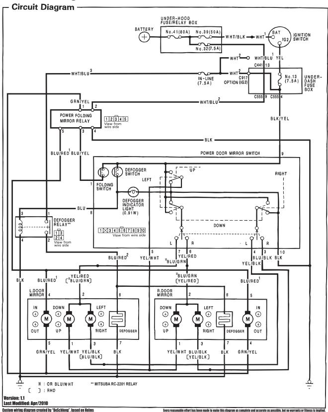
Custom wiring diagram created by "DeSchlong", based on Helms manuals for EDM 1992-1995 Honda Civic & CDM / USDM 1991-1995 Acura Legend, and original PFM diagram posted on Honda-Tech.com by user "Jacob".
